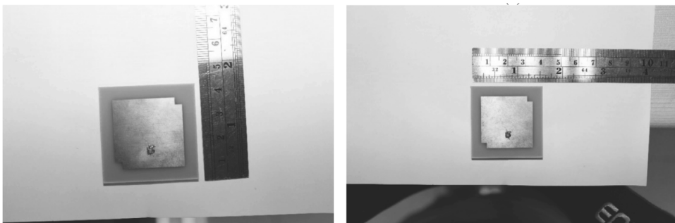
Fig. 8. Prototype of the antenna after fabrication from two different views
